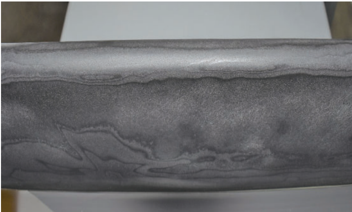
✔ Newly applied DSX leading edge coating to an OH-58 main rotor blade.
